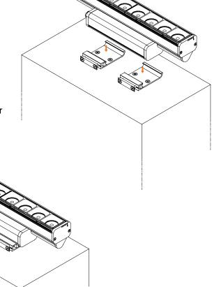
Tighten the screw on the side of the brackets to fix the profile.
