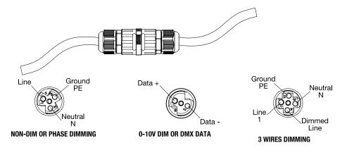
For 0-10v dimming, the fixture are provided with two (2) cable leads, one with a 3 pin connector for power and the other with 2 pins connector for dimming wires. follow below connector labeling for termination of wires.
