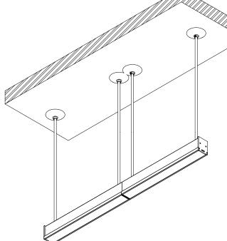
WARNING: Do not exceed the rated wattage of the through wiring cables or the connectors. For all continuous runs, refer to factory shop drawing indicating exact dimensions and feed locations.
