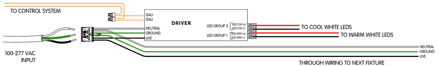
**2 CHANNELS 0-10V WIRING DIAGRAM**
