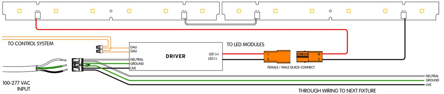
**0-10V WIRING DIAGRAM**
