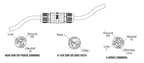
For 0-10v dimming, the fixture are provided with two (2) cable leads, one with a 3 pin connector for power and the other with 2 pins connector for dimming wires. follow below connector labeling for termination of wires.
