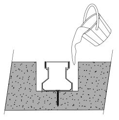
Housing spacer should be used during installation to avoid housing apreture being deformed by accident.
